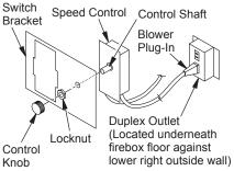
Figure 26 - Attaching Speed Control to Firebox
